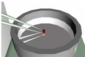
Fig. 3 Micro gripper and its mirror image on the aluminium coated specimen holder
