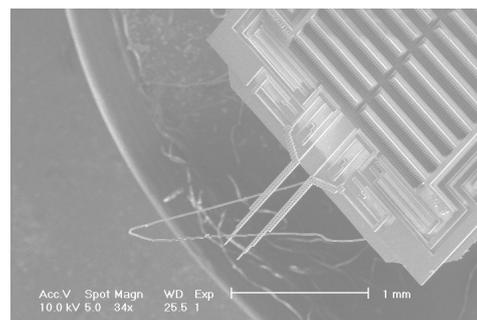
Fig. 2 Wire 10 µm on the specimen holder
