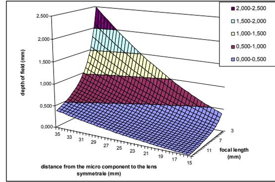
Fig.5 Depth of field depending on the focal length of the lens and the distance micro camera-micro component
