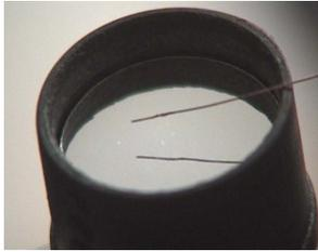
Fig. 7 Wire 50 μm, and its image on the aluminium coated specimen holder
