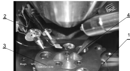
Fig. 1 View of the CCD camera inside the SEM chamber.
