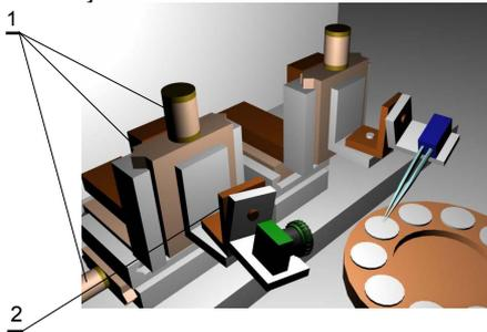
Fig. 8 Micro camera mounted on the tweezers module
