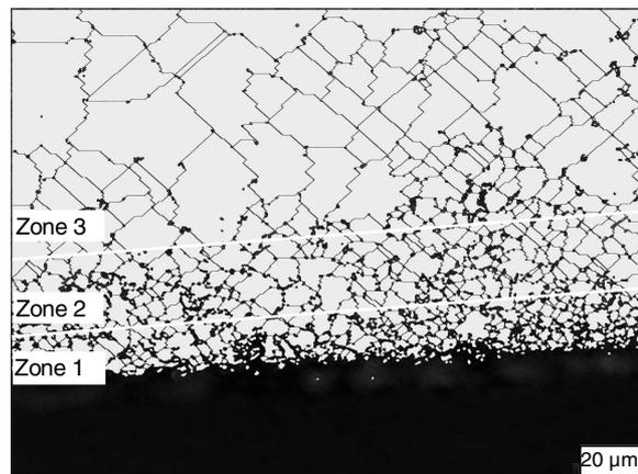
Figure 2 A micrograph depicting the three characteristic zones after machining with ps laser
