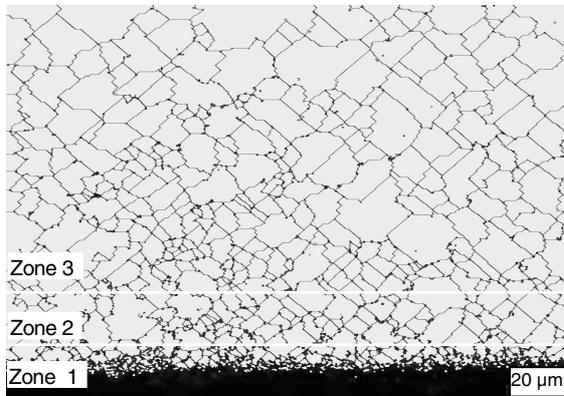
Figure 3 A micrograph depicting the three characteristic zones after machining with fs laser
