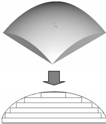
Fig. 2 The 3D CAD model created with ProEngineer and a schematic representation of the sliced model in N layers.
