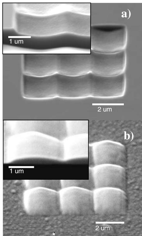
Fig. 3. SEM images at  $36^\circ$  of  $3 \times 3$  arrays of square lenses produced employing layer-based FIB processing: a) sputtering and b) Pt gaseous precursor assisted GA deposition.
