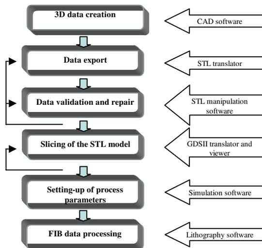
Fig. 1 The key steps of the proposed CAD/CAM method for layer-based FIB processing
