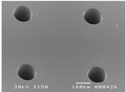
Fig.1 Laser trepanned holes in silicon using high intensity (15 GW/cm<sup>2</sup>) at 355nm.
