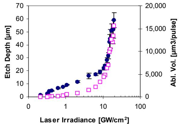
Fig.3 Single-shot etch depth (solid circle) and ablated crater volume (open square) measurements of crystalline silicon as a function of incident laser irradiance at 355nm.
