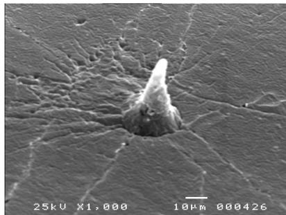
Fig.2 SEM of a negative imprint of a single-shot laser ablation crater in silicon using 355nm at 19 GW/cm<sup>2</sup>.
