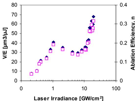
Fig.4 Ablation volume per unit input energy ( $V/E_p$ ) (solid diamonds) and ablation efficiency (open square) as a function of incident laser irradiance at 355nm.
