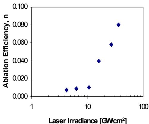
Fig.6 Ablation efficiency of stainless steel as a function of incident laser irradiance at 532nm.
