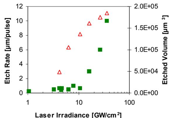
Fig.5 Average etch rate (solid square) and ablated volume (open triangle) in stainless steel as a function of incident laser irradiance at 532nm.
