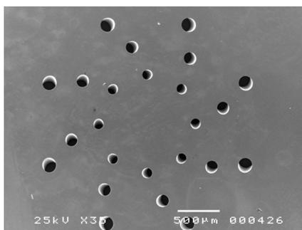
Fig.7 High aspect ratio laser drilling of a stainless steel fuel-injection nozzle.
