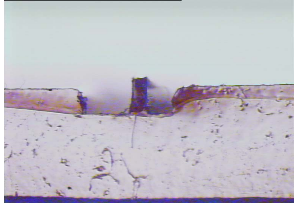
Fig. 3. Cross section of hot embossed waveguide fabricated in Topas® grades 8007 (substrate) and 9506 (core). The waveguide is the dark rectangle in the middle surrounded by air from both sides. The dimensions of the waveguide are approximately 120 \mu\text{m} \times 200 \mu\text{m} .
